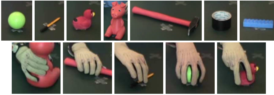
Fig. 3. Top row: the objects used in our experiments. Bottom, the grasp types we consider: (left to right) cylindrical power grasp, flat grasp, pinch grip, spherical and tripod grasp.
