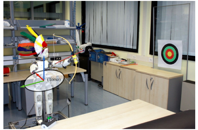
Fig. 7. Real-world experiment using the iCub [14]. The distance between the target and the robot is 2.2 meters. The diameter of the target is 50 cm.
