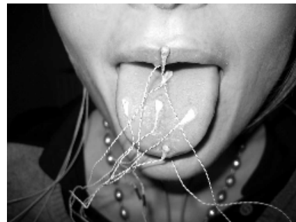
Figure 1: EMA sensors glued on the subject's tongue
