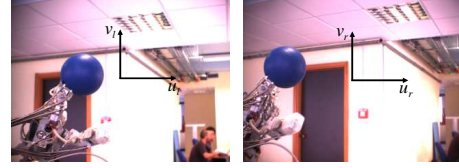
Fig. 2. Two typical images taken from the two cameras mounted on the eyes of the robot (resolution 320 \times 240 ). The coordinates of the target (the blue ball) on the image planes will be denoted u_r , v_r , and u_l , v_l (respectively right and left cameras).
